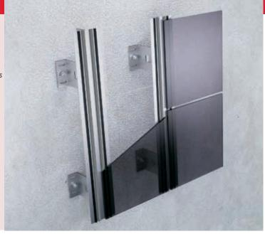
Aluminium substructure system for flat panel cladding featuring invisible mounting with glue. This wet installation method requires preparation both in workshop and on construction site. It offers great flexibility with cladding material options, facade design and unusual aesthetics with numerous possibilities for combining of irregular shapes and forms on the facade.
