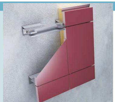
Aluminium substructure system for specially machined and shaped cassettes. Their installation is extremelly easy due to easy matching of two specially constructed aluminium profiles that fit perfectly together. It's trademark are fine visible gaps, only 9mm wide, and if underlying profile is powder coated the gap can even be colored. This dry installation system features partial workshop preparation and quick installation.
