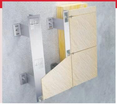
Aluminium substructure system for flat panel cladding (usually granite ceramic) fixed by stainless steel cleats with visible or hidden fixing system. The visible part of the stainless steel cleat can be powder coated in any RAL color according to project requirements. This dry installation system features simple installation, high load-barring capacity which makes it the industry standard for heavy cladding materials.
