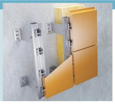
Aluminium substructure system for specially machined and shaped cassettes fixed by sliding panel brackets with visible bolts in gaps between cassettes. This dry installation system features quick and efficient installation due to complete workshop preparation of all cassettes. It is named after fixing method after special sliding brackets that are fixed to each cassette and later slide onto load-barring substructure.
