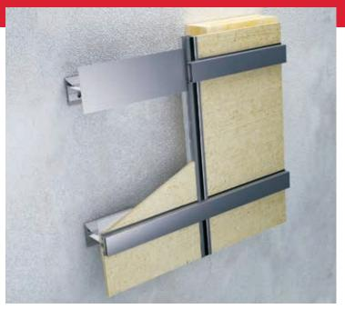
Aluminium substructure system for flat panel cladding featuring emphasized visible facade partitions. This partitioning is possible via vertical and horizontal cover caps, in all according to architect's proposal. This way, the the same visual effect as with glass curtain walls achieved is (therefore the system's name Continual). This dry installation system has no limits regarding the cladding panel material.
