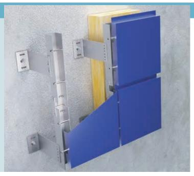
Aluminium substructure system for specially machined and shaped cassettes fixed by panel brackets with visible bolts in gaps between cassettes (this is where the system's name comes from). This dry installation system features specially machined openings used to fix cassetess for aluminium substructure.
