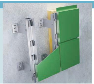
Aluminium substructure system for installation of specially machined and formed cassettes fixed with hidden cantilevers and brackets formed from small square tube profiles. This dry installation system features full workshop preparation of cassettes that are quickly installed on a construction site as finished facade elements.
